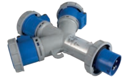
Ref. 904015 Clavija industrial + 3 bases industriales. 2P+T, 16A 230V. IP67.
