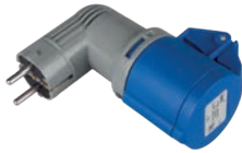
Ref. 904011 Clavija doméstica schuko + base industrial. 2P+T, 16A 230V. IP44.
